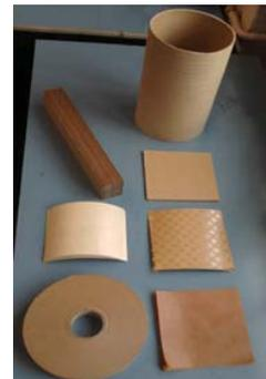
Fig. 1 Different types of transformers insulation material
