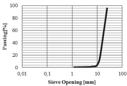
Fig. 2 Gravel grading
