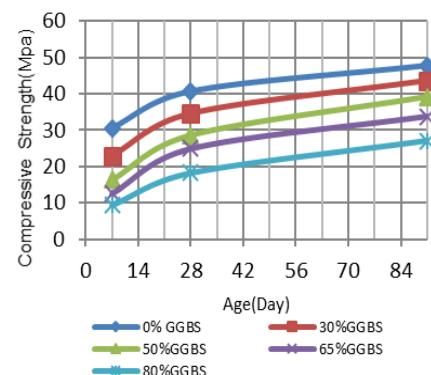
Fig. 12 Compressive strength development of RCC by ages
