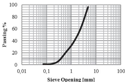
Fig. 1 Sand grading
