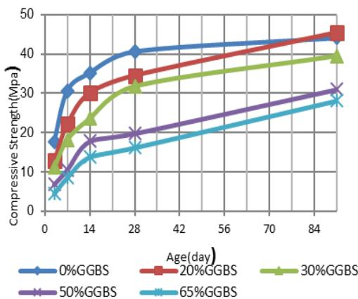
Fig. 11 Compressive strength development of NC by ages
