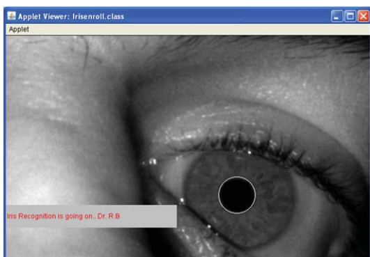
Fig. 4 Depiction of Inner boundary detection and Occlusion of eyelashes/eyelids on the iris Patterns
