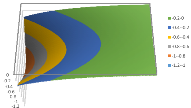
Fig. 11 Axisymmetric nozzle theoretical pressure p ( 0 \leq z \leq 1.3, 0 \leq r \leq 2 )
