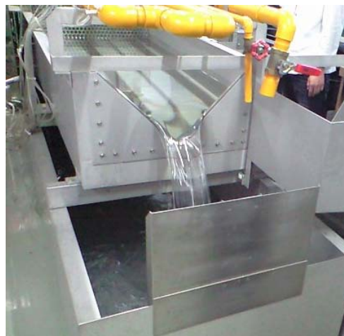
Fig. 2 Regular triangular weir of 320 mm side length
