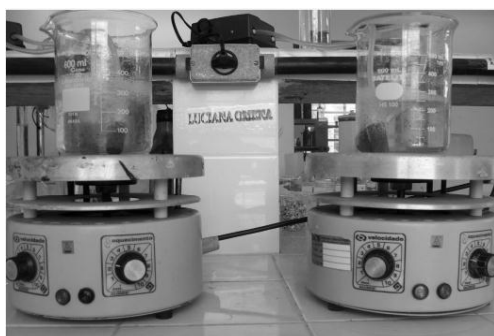
Fig. 1 Experimental set-up of the flotation process used to treat produced water
