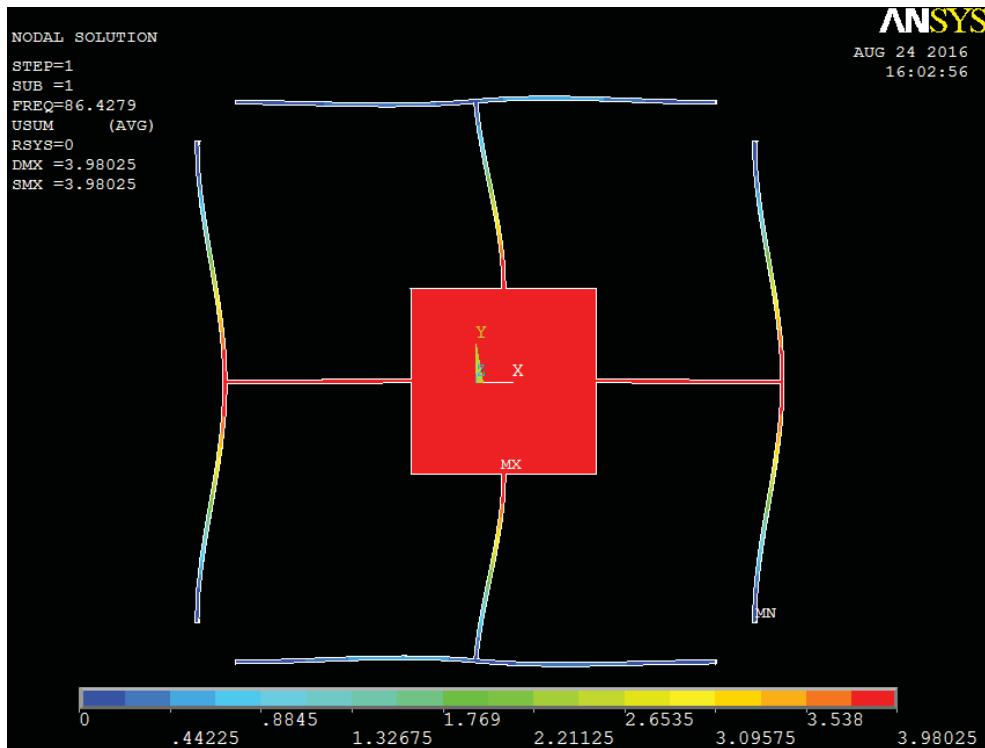
Fig. 5 ANSYS finite element simulation of the relative displacement for the two vibration modes when only one mode is vibrating, it is clear that the vibration of one mode does not have a significant effect on the other mode
