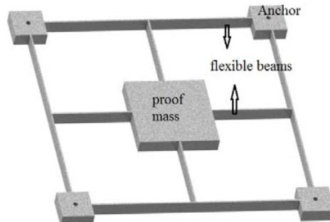
Fig. 1 Symmetrical single mass resonant gyroscope design
