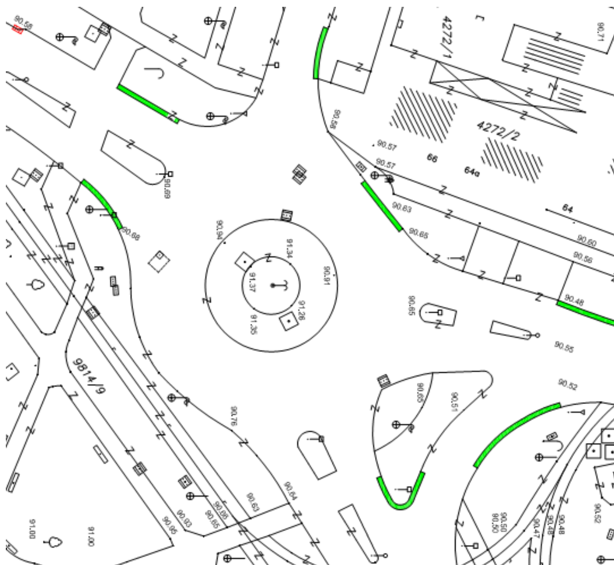
Fig. 5 Potential application of pervious concrete on a small urban roundabout
