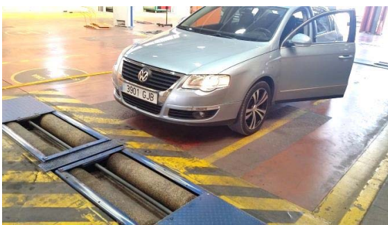
Fig. 2 Vehicle on the brake roller tester at the MOT centre of Elche
