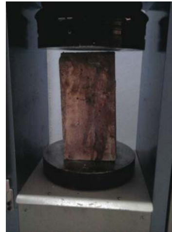
Fig. 6 A corroded column specimen before compressive testing
