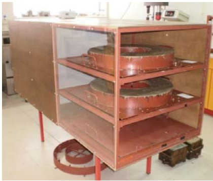
Fig. 2 Cracking specimens in the wind tunnel
