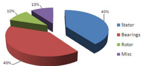
Fig. 1 IM faults distribution by zone [1]
