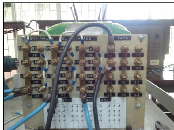
Fig. 5 Connection board of the motor under test
