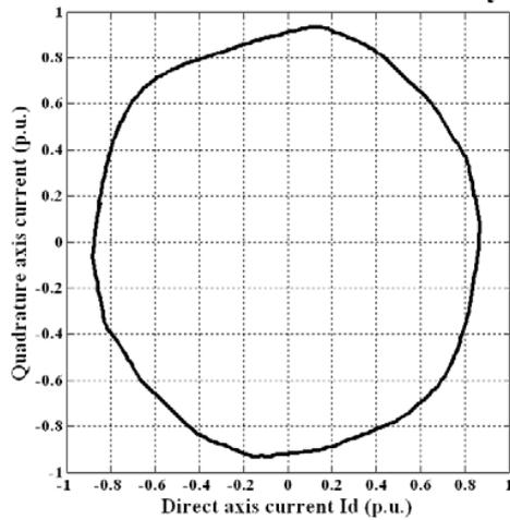
Fig. 13 Park's vector representation (p.u.) in Gaussian plane for healthy condition
