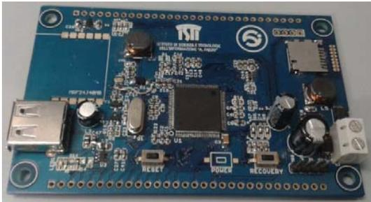
Fig. 8 The smart camera main electronic board
