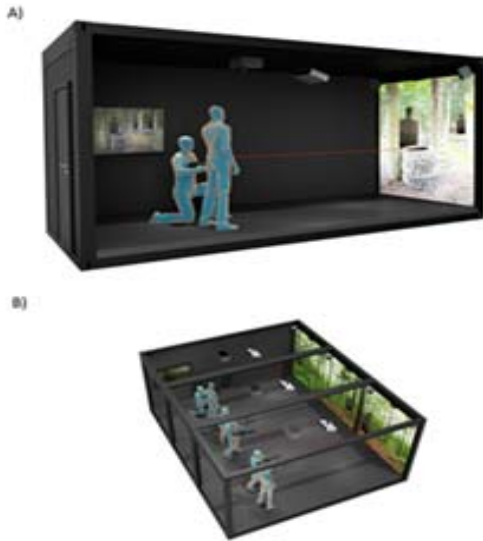
Fig. 1 The system architecture enables modular use of the system (A) a single track, (B) multiple tracks simultaneously
