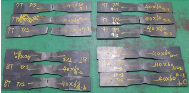
Fig. 3 Fracture of tension coupon test result
