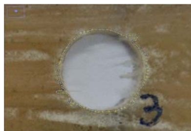
Fig. 4 Delaminated hole for hole 3
