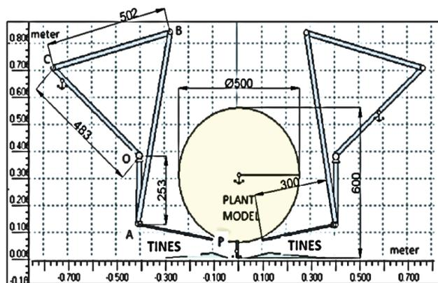
Fig. 9 The plant body model and four-bar mechanism
