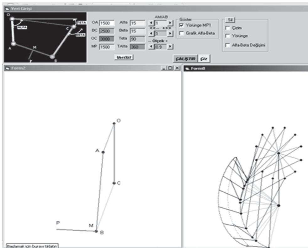
Fig. 4 Four bar linkage trajectory simulation software
