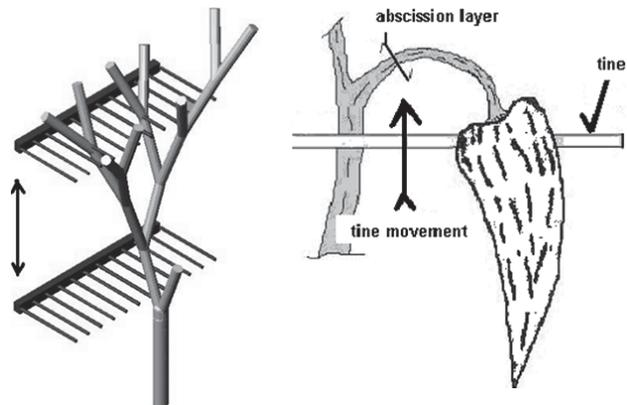
Fig. 8 Principle of pepper removal by tine
