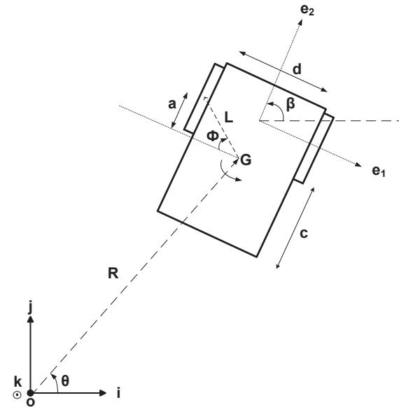
Fig. 1 Schematics of the differential drive robot [13], [28]
