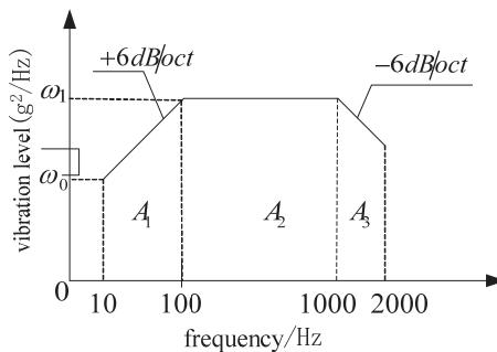
Fig. 11 The test control spectrum of Random vibration
