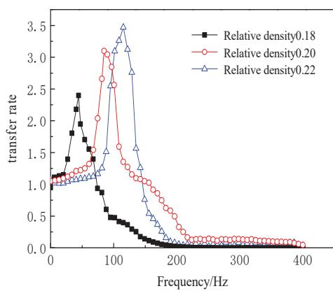
Fig. 7 Transfer rate-frequency curve of different relative densities
