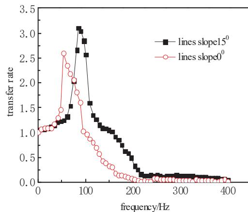
Fig. 5 Transfer rate-frequency curve of different lines slope
