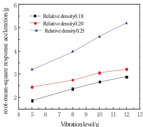
Fig. 13 Relationship between root-mean-square response acceleration and vibration level under different relative densities
