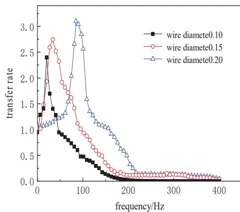
Fig. 9 Transfer rate-frequency curve of different wire diameters
