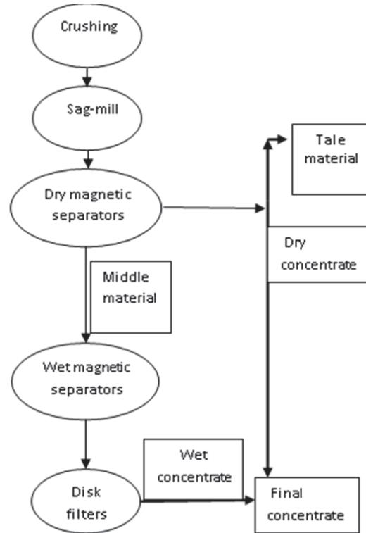
Fig. 1 Schematic presentation of iron Concentration Plant
