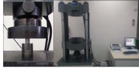
Fig. 4 Hydraulic Press and fixation of parts
