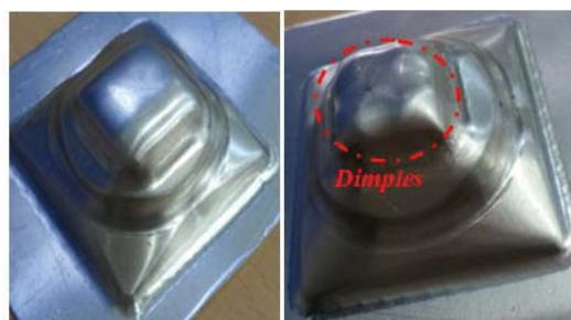
Fig. 7 Influence of the elastomeric interpolator
