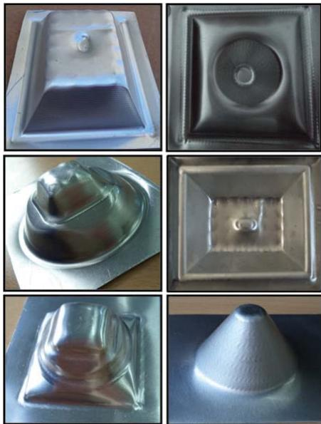
Fig. 3 Parts manufactured using the MPIF process
