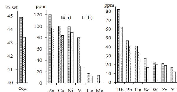
Fig. 1 The organic matter content ( $C_{\text{org}}$ ) and ore elements change in the kukersite oil-shales: a) initial content of the elements in the oil-shales before experiment's start; b) content of the elements after experiment
