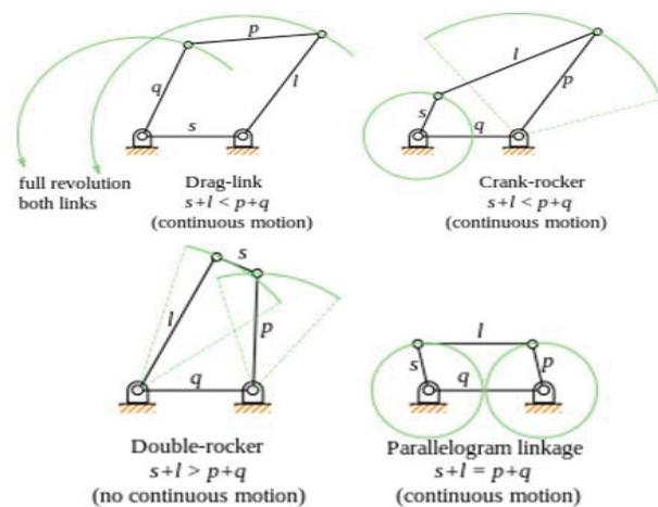
Fig. 2 The 4BL Mechanisms according to Grashof [11], [14]
