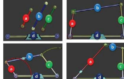
Fig. 3 (a) Linkage Parts. (b) Drag-Link. (c) Double-Rocker (d) Crank-Rocker (e) Parallelogram-Linkage (f) Dynamics of the Crank-Rocker
