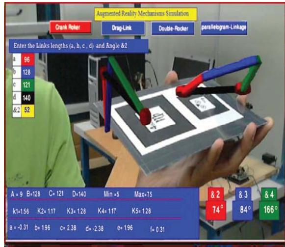
Fig. 5 A programmable simulation of the 4BL mechanism
