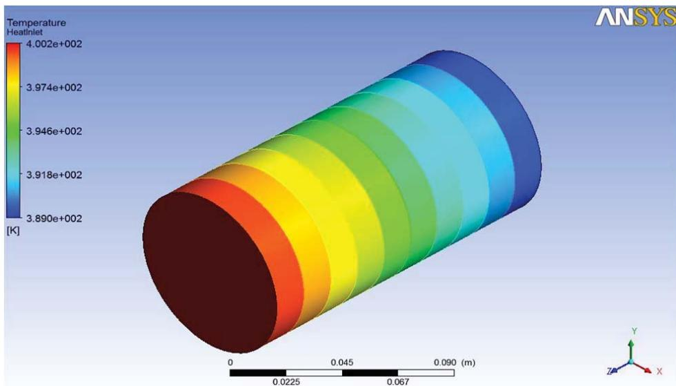
Fig. 4 Temperature distribution along a discrete Extrudate in 3-dimension
