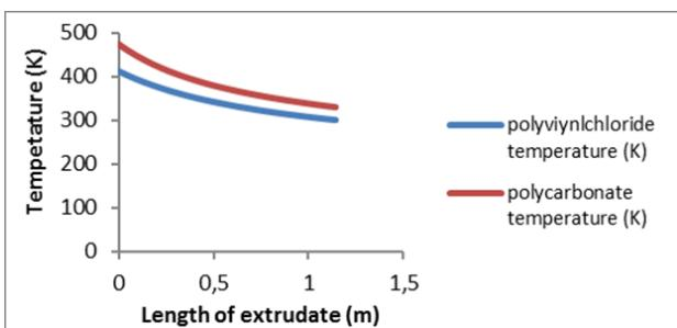
Fig. 2 Temperature distribution and extrude length of the plastics employed
