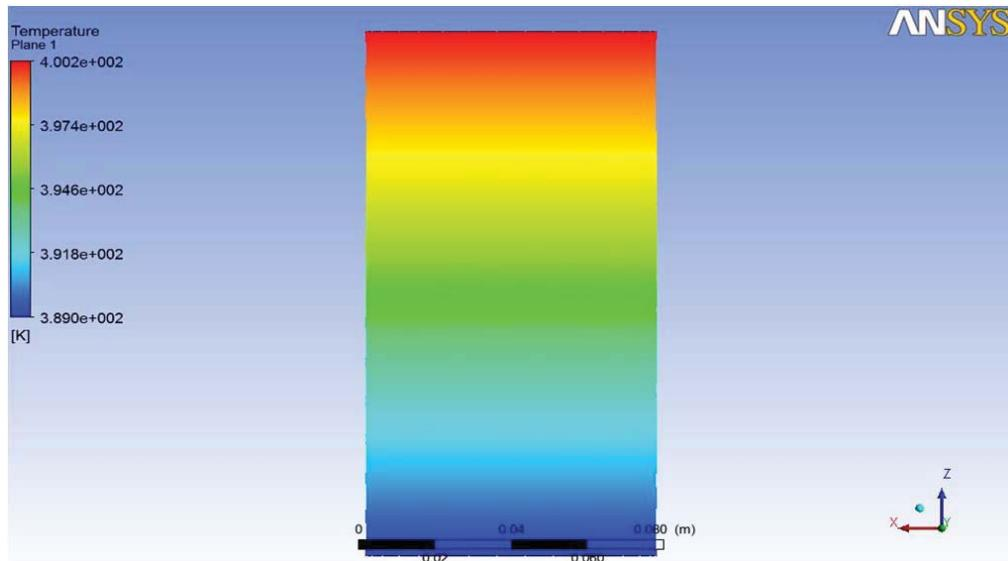
Fig. 5 Temperature distribution along an Extrudate in 2-dimension
