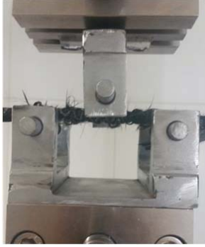
Fig. 7 A non-crimp 3D orthogonal carbon specimen subjected to three-point bending test
