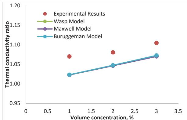
Fig. 12 Comparison of the measured thermal conductivity ratio of the NiFe<sub>2</sub>O<sub>4</sub>/water nanofluids with the well-known correlations
