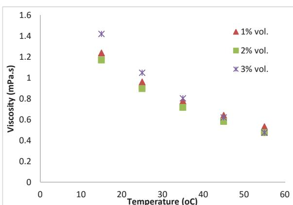
Fig. 13 Viscosity variations of pure water and NiFe<sub>2</sub>O<sub>4</sub>/water nanofluids with temperature for different volume concentrations
