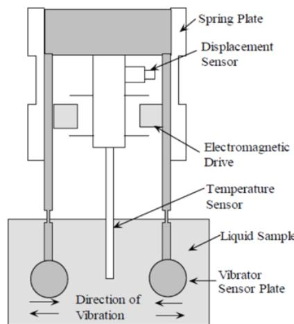
Fig. 3 A schematic diagram of Vibro Viscometer [25]
