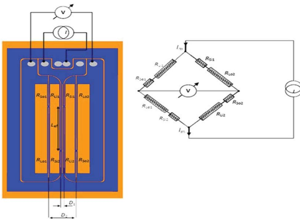
Fig. 1 THB6K sensor and equivalent electrical circuit diagram [24]
