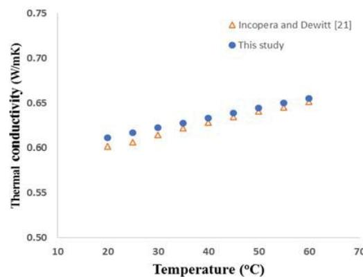
Fig. 4 Comparison of the thermal conductivity data for pure water with [26]
