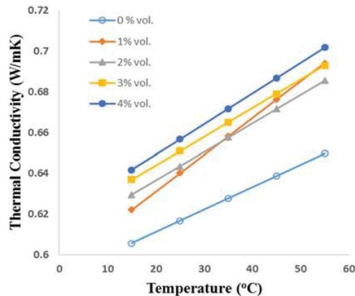
Fig. 6 Thermal conductivity variations of pure water and CoFe<sub>2</sub>O<sub>4</sub>/water nanofluids
