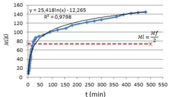
Fig. 3 Aging of the foam over time
