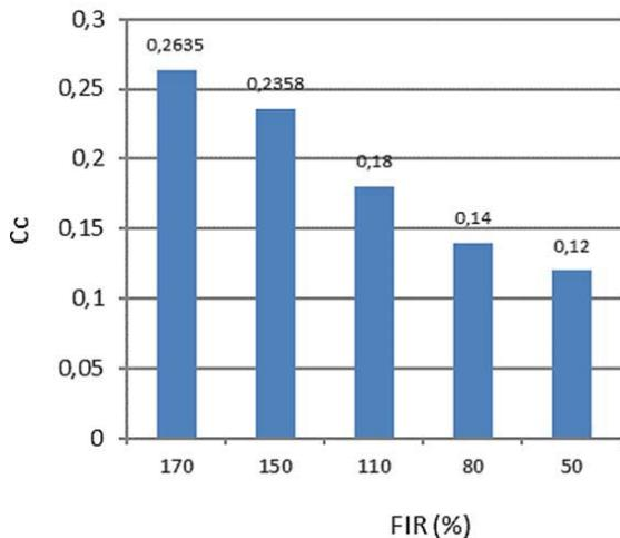
Fig. 7 Compression index variation depending on the FIR
