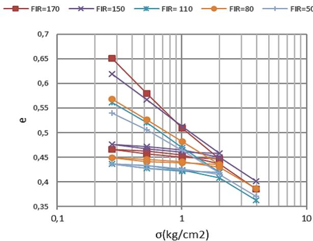
Fig. 5 Compression curve of untreated soil FIR (%)
