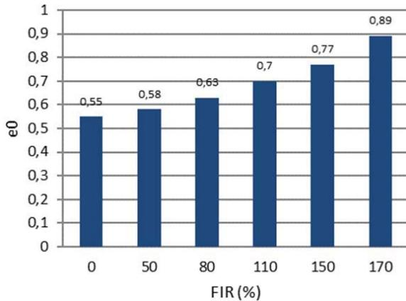
Fig. 6 Void ration variation depending on the FIR
