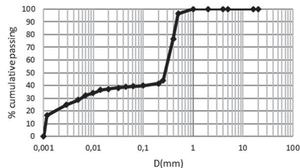
Fig. 1 Graduation curve of model soil
