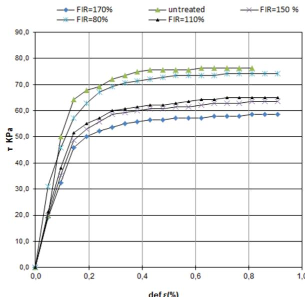
Fig. 9 Curves shear stress vs. horizontal deformation with different FIR ( $\sigma_N=148 \text{ kPa}$ )
