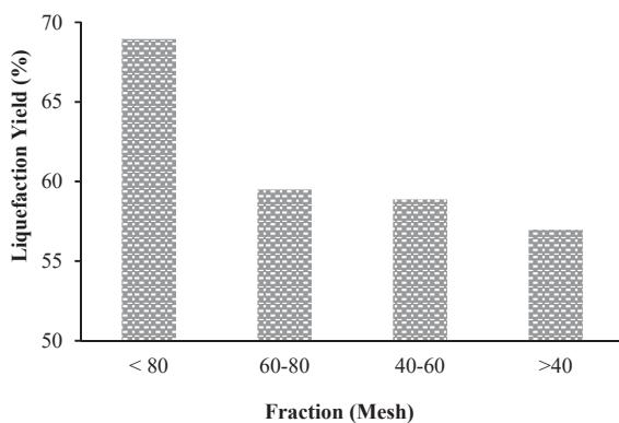
Fig. 1 Liquefaction yield (%) with fraction (mesh) for cork
