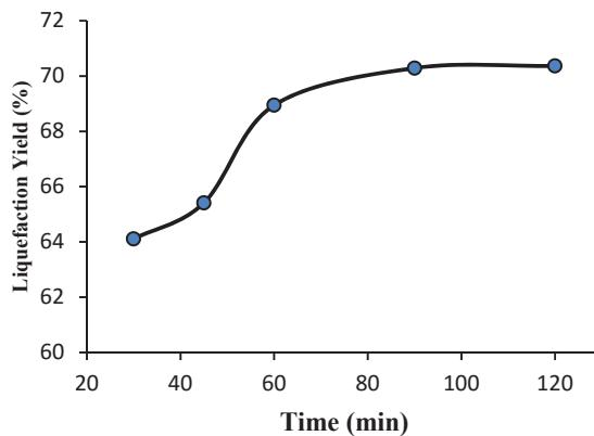
Fig. 3 Liquefaction yield (%) with time (minutes) for cork
