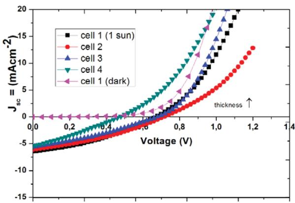
Fig. 5 J-V measurements of different cells w.r.t thickness (perovskite film consist of 1wt% DI-H<sub>2</sub>O)
