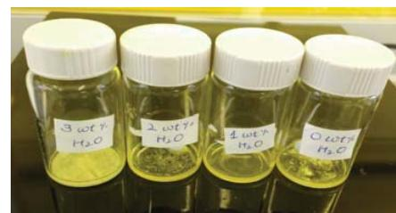
Fig. 2 Photograph of DMF/PbI<sub>2</sub> precursor solutions consisting of various amounts of additive DI-H<sub>2</sub>O
