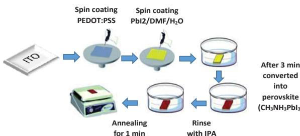
Fig. 1 Schematic illustration of the sequential deposition process
