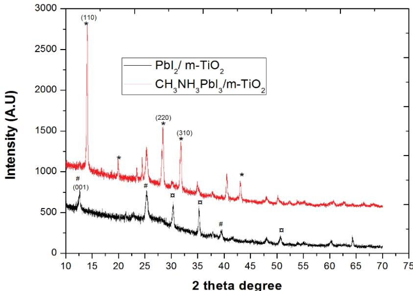
Fig. 4 XRD pattern of  $\text{PbI}_2$  (black) and  $\text{CH}_3\text{NH}_3\text{PbI}_3$  (red) films. The major peaks are from  $\text{PbI}_2$  (#),  $\text{CH}_3\text{NH}_3\text{PbI}_3$  (\*) and FTO/mTiO<sub>2</sub> substrate. (□)
