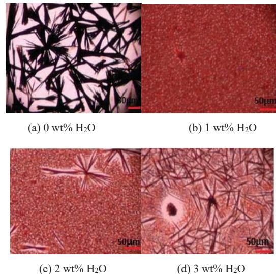
Fig. 3 Optical images of perovskite films consisting of various amounts of DI-H<sub>2</sub>O in PbI<sub>2</sub>/DMF solution (DI-H<sub>2</sub>O content is wt% ratio vs DMF)
