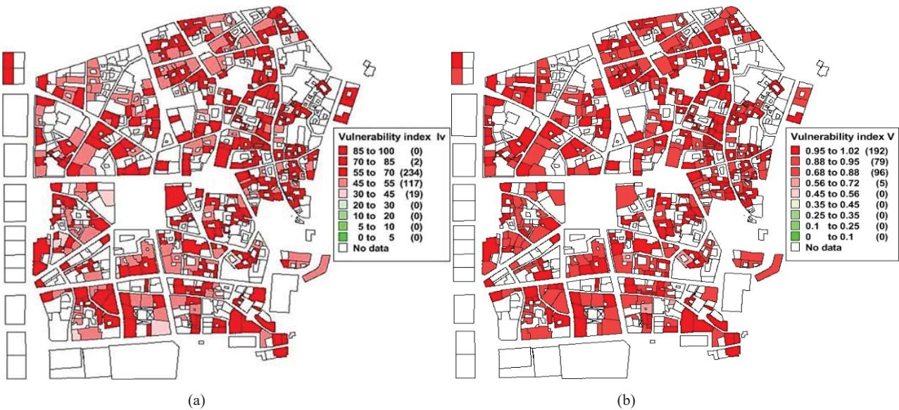
Fig. 5 Vulnerability distribution: (a)  $I_v$  according to the modified GNDT level II; and (b)  $V$  according to the modified RISK-UE
