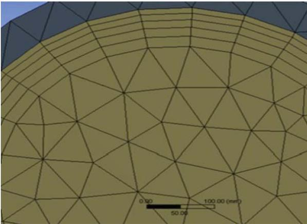
Fig. 3 Inflation on boundary of solid and fluid
