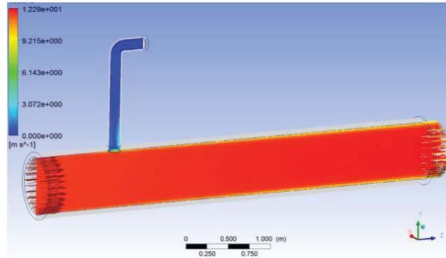
Fig. 4 Velocity distribution in Type I pipe
