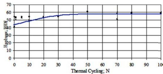
Fig. 3 Effect of thermal fatigue on hardness at temperature; T<sub>h</sub> =100°C
