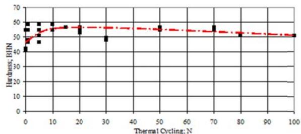
Fig. 4 Effect of thermal fatigue on hardness at temperature; T<sub>h</sub>=300 °C
