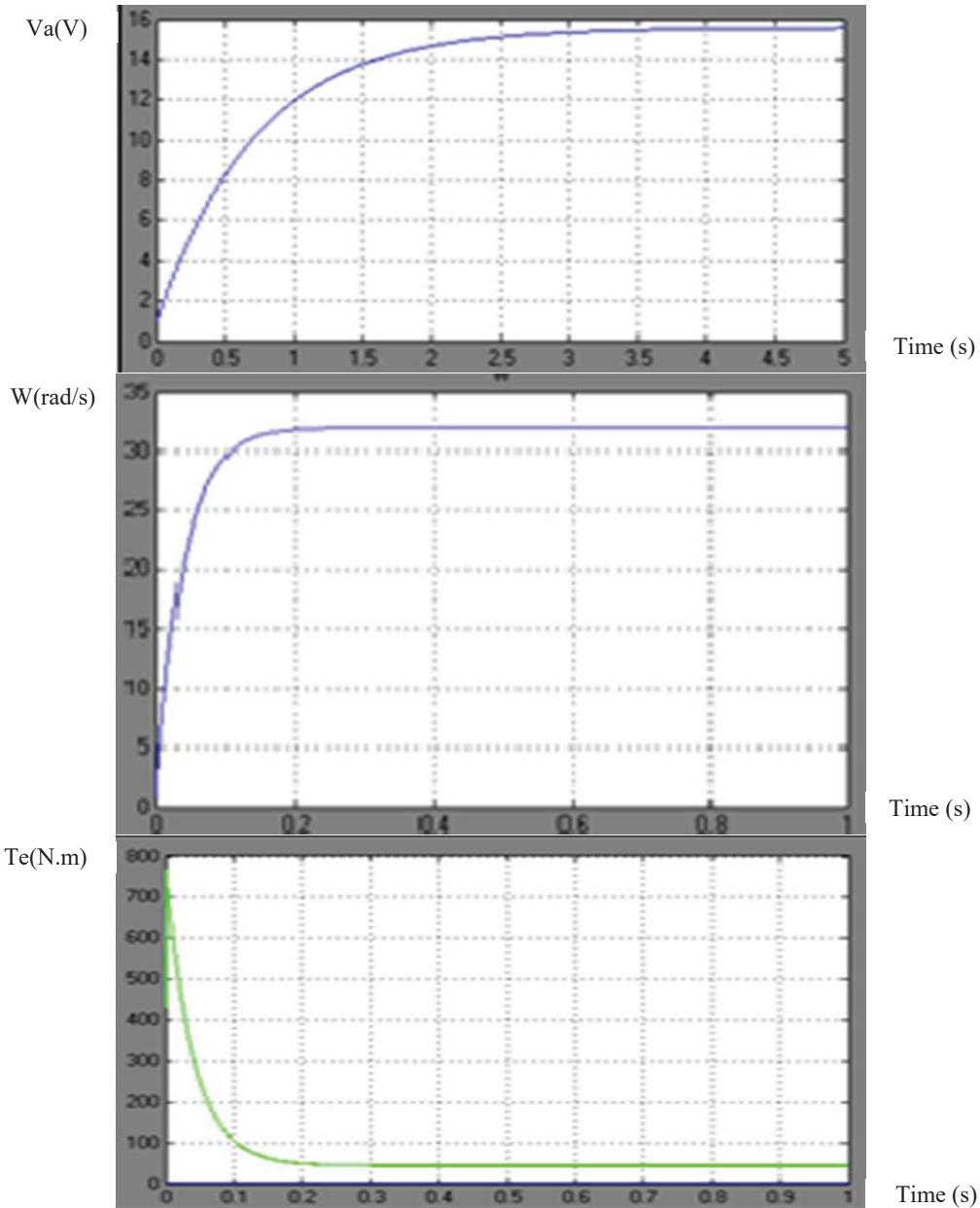
Fig. 6 Simulink output of DC motor characteristics
