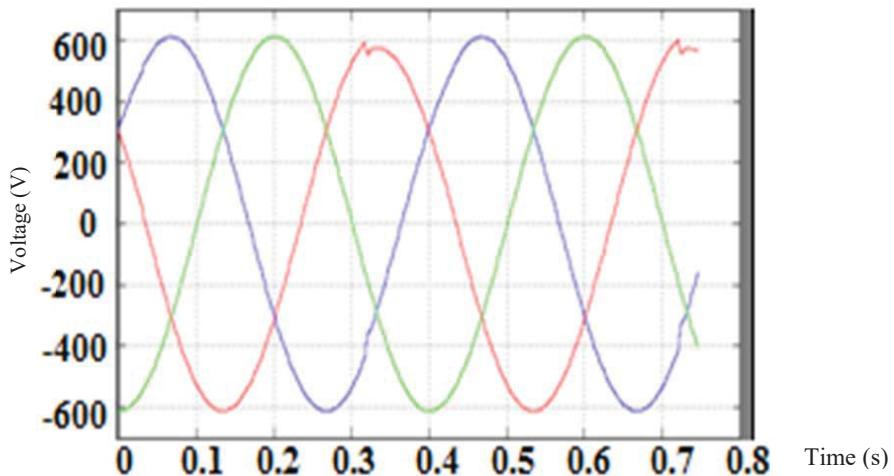
Fig. 8 Simulink result of output characteristic of the inverter
