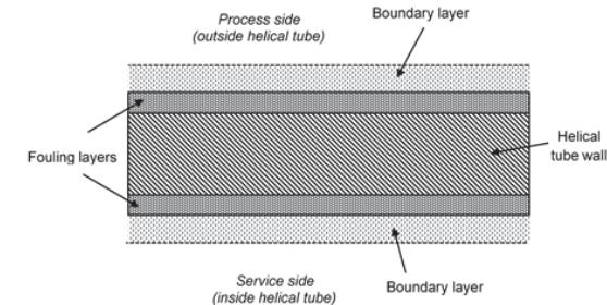
Fig. 2 Thermal resistances through the helical tube wall sections
