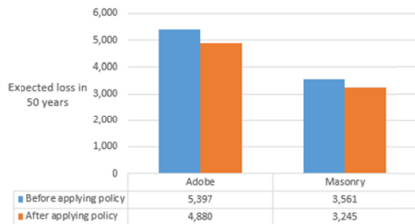
Fig. 22 A comparison of the reduction in expected loss of lives for nighttime earthquake scenario
