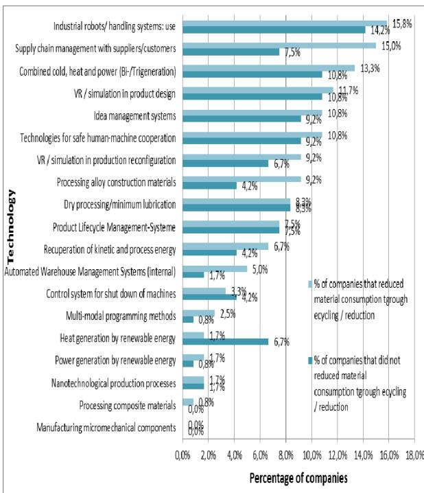
Fig. 2 Technologies for material savings by recycling
