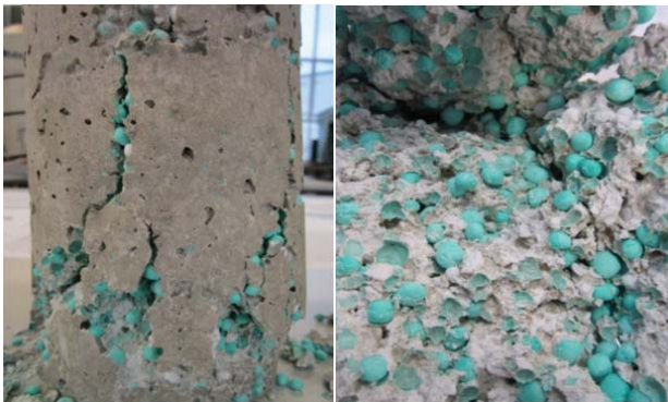
Fig. 4 Failure modes of PLA concrete
