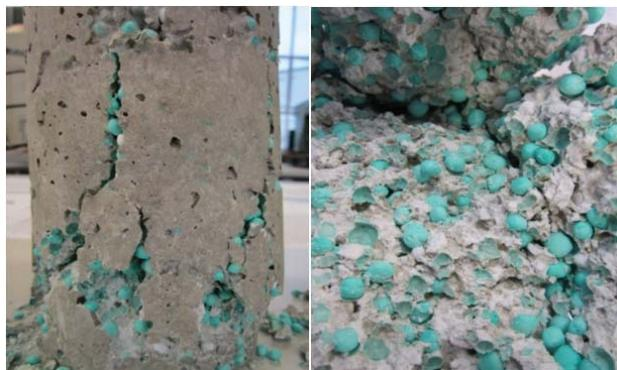
Fig. 4 Failure modes of PLA concrete
