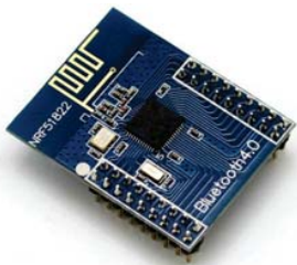
Fig. 7 Minimum working development BLE module nRF51822 SoC
