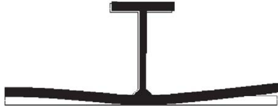
(b) Schematic view of the Angular distortion in the stiffened cylinder in the first method
