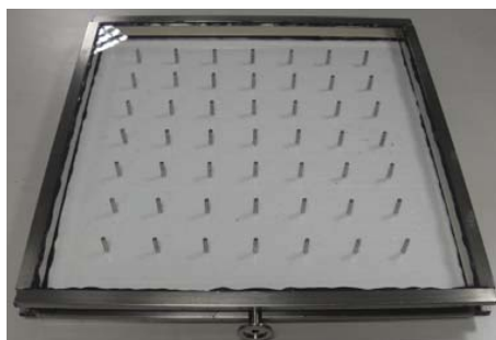
Fig. 9 Fabricated flat vacuum panel
