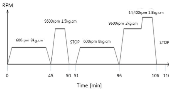
Fig. 3 The operating cycle profile of washing machine
