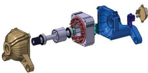
Fig. 2 Structure of BLDC Motor for Washing machine
