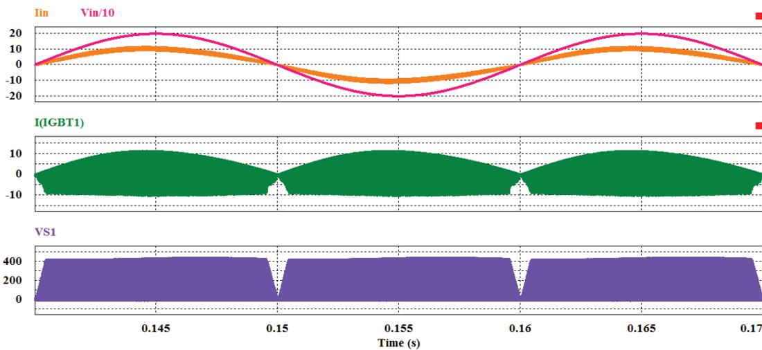
Fig. 8 Respectively; the input voltage and current waveforms of PFC converter, the current waveform and the voltage waveform of the main switch
