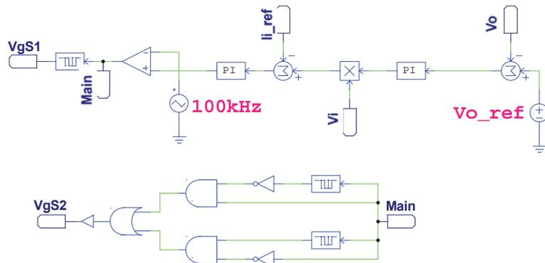
Fig. 3 PFC average current control block scheme for PWM control signals
