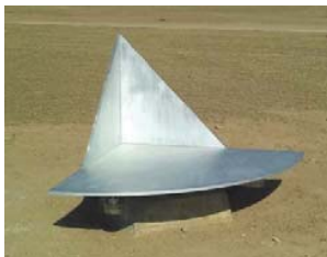
Fig. 5 The bottom-extended trihedral CR deployed in the National Calibration and Validation Site for High Resolution Remote Sensors
