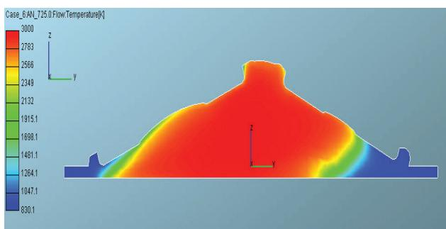
Fig. 7 Spatial distribution of temperature in y-z plane,  $x=\text{const.}$  at 365 deg. ATDC,  $k-\epsilon$ , C8H18
