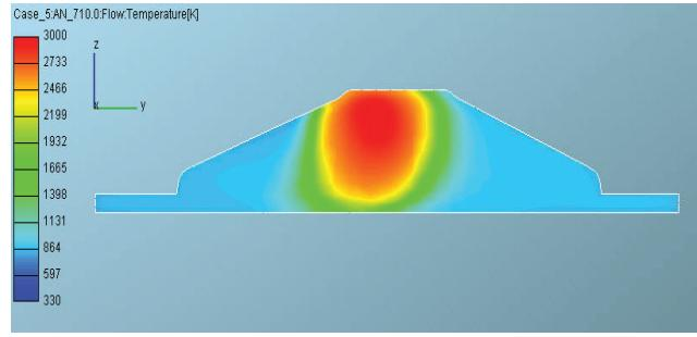
Fig. 14 Spatial distribution of temperature in y-z symmetry plane,  $x=0.0$  at 350 deg. ATDC,  $k-\epsilon$ , CH4
