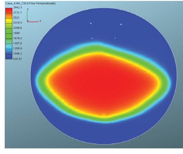
Fig. 27 Spatial distribution of temperature in x-y plane passing through squish zone at 360 deg. ATDC, k- $\epsilon$ , C8H18
