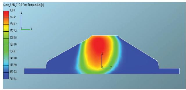
Fig. 13 Spatial distribution of temperature in y-z symmetry plane,  $x=0.0$  at 350 deg. ATDC,  $k-\epsilon$ , C8H18
