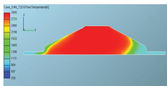
Fig. 20 Spatial distribution of temperature in y-z symmetry plane,  $x=0.0$  at 365 deg. ATDC, k- $\epsilon$ , CH4
