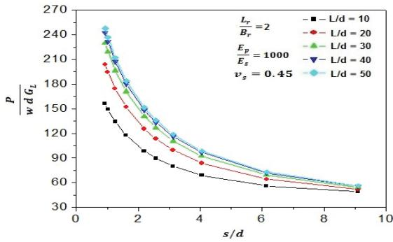
Fig. 4 Piled Raft Stiffness for  $\frac{E_p}{E_s} = 1000$ ,  $v_s = 0.45$ , and  $\frac{L_r}{B_r} = 2$
