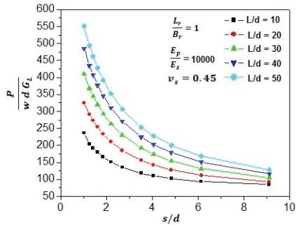
Fig. 5 Piled Raft Stiffness for  $\frac{E_p}{E_s} = 10000$  and  $\frac{L_r}{B_r} = 1$
