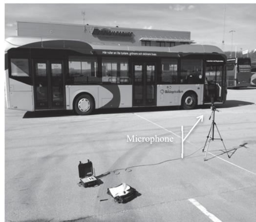
Fig. 5 Compressed air noise measurements of the hybrid bus. Photo:
