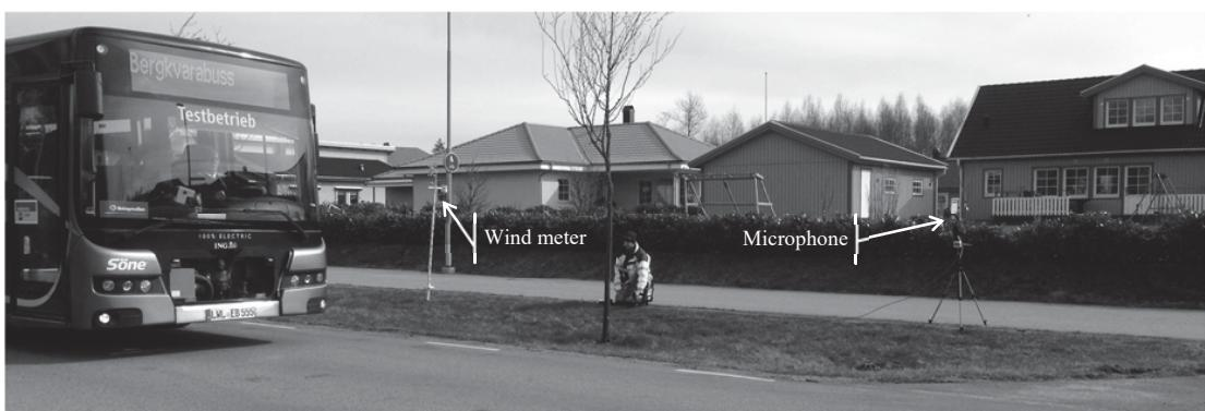
Fig. 2 Noise measurement of the electric bus when driving 30 km/h. Photo: Sven Borén
