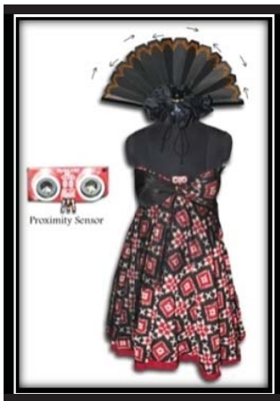
Fig. 4 Black Ikat print Interactive garment integrated with proximity sensors, servo motor
