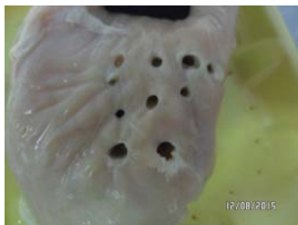
Fig. 7 Various void sizes in chicken breast created by varying the frequency of the modulating signal: higher frequencies generated smaller void diameters
