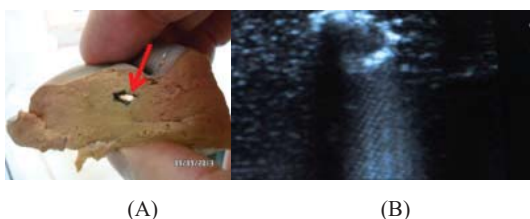
Fig. 8 (A) Bovine liver section showing void remaining after fractionated tissue (arrow). (B) The image of the void on a B-mode ultrasound scanner
