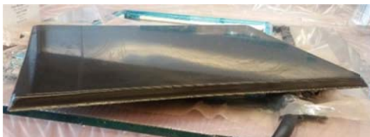
Fig. 2 Core sheets with 3% Boron Nano powder
