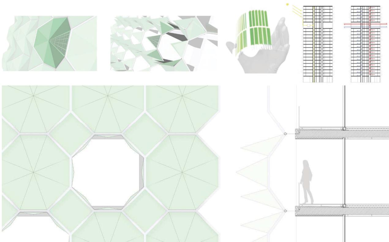
Fig. 15 Octagonal module, each using 8 flectofin-shading-elements [10]
