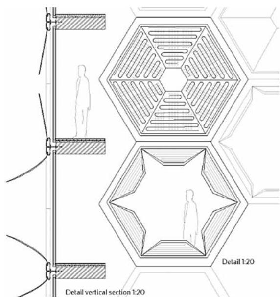
Fig. 19 Honeycomb – structure for shading-device element [11]
